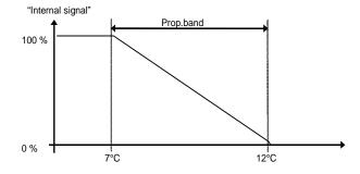
The frost protection signal ("Internal signal") will increase linearly to 100 % at 7°C at which point the frost protection alarm is triggered. The fan will then be shut down and the controller will go into shutdown mode.
