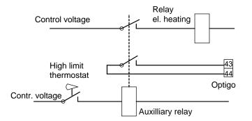
Wiring suggestion for high temp limit when using electric heating. Drawn with high temp. limit activated.
