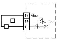
In OP10-230 however, the internal transformer's capacity restricts the current on  $G_{\text{DO}}$  to approx. 165 mA.
