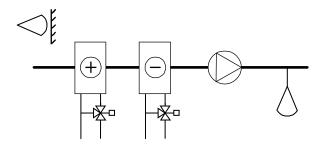
For control mode 3, "Cascade connected room / extract air temperature control" you also need 2 sensors, "Supply air sensor" on AI1 and "Room sensor", which are placed in the room or in the extract air on AI2.
