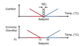
The above schematic drawings of the control principle show the corresponding requirement of the controller function. This requirement is recalculated by the controller to a value for the actuator output, depending on the selected output function.
