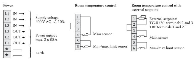
NOTE: When controlling Y-connected loads, the load must be symmetric and the signal neutral must not be connected!
