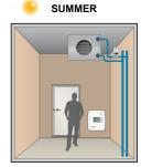
In 4-pipe installations, there are two separate pipe systems for heating and cooling with separate valves. The controller uses two outputs for control of heating and cooling in sequence with two thermal actuators.
