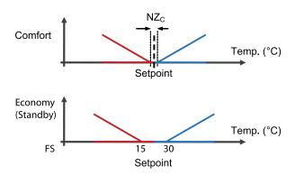
The above schematic drawings of the control principle show the corresponding requirement of the controller function. This requirement is recalculated by the controller to a value for the actuator output, depending on the selected output function.
