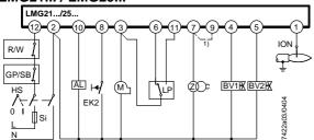
1) Wire link required only with the LGB21..., not with the LMG21... / LMG25...
