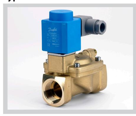
EV224B is a high pressure indirect servo-operated 2/2-way solenoid valve with working pressure up to 40 bar, medium temperature up to 60 °C and available in NC and NO versions.
