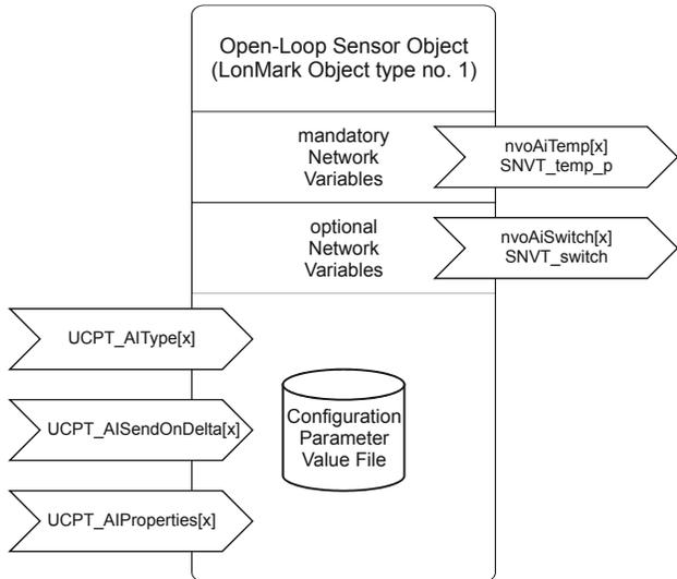
Fig. 7. Profile of LONMARK sensor objects for UIs
