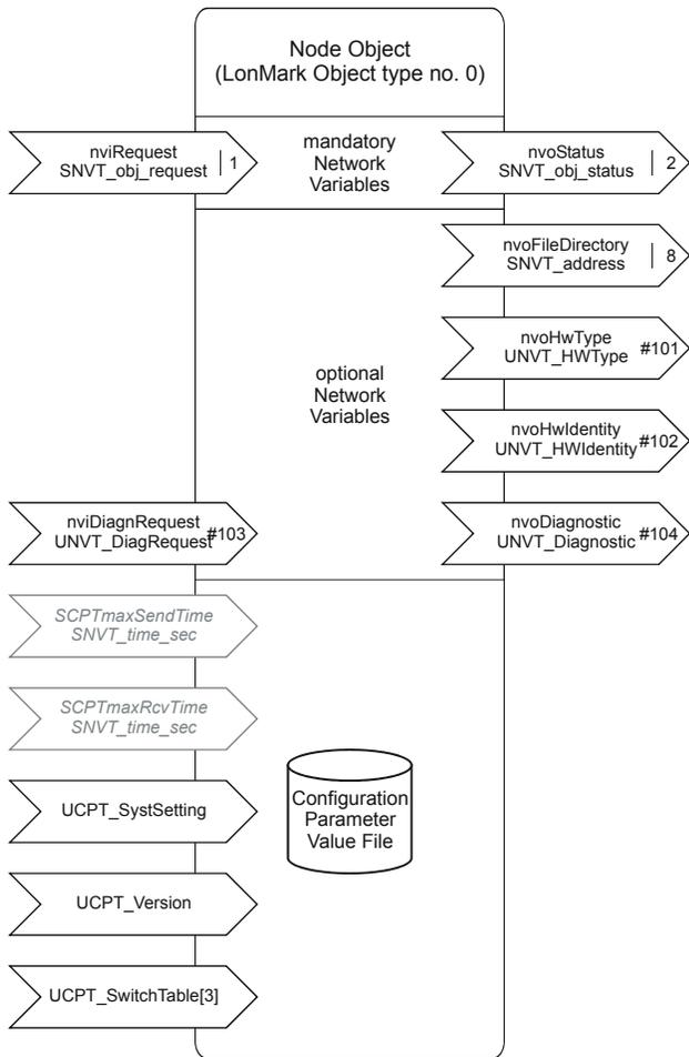
Fig. 6. Profile of LONMARK node object
