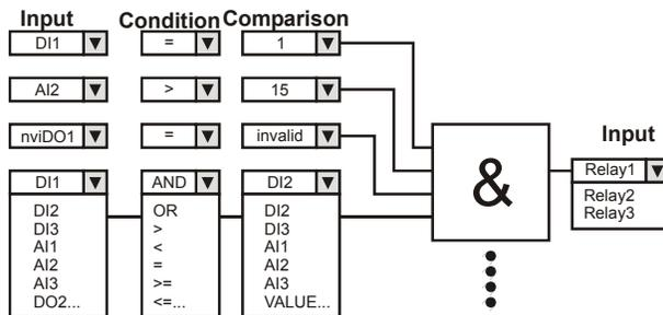
Fig. 1. Switching logic functionality
