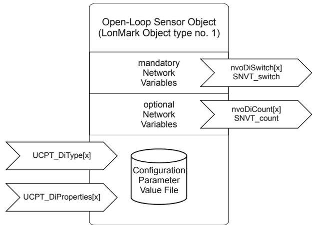
Fig. 8. Profile of LONMARK sensor objects for DIs
