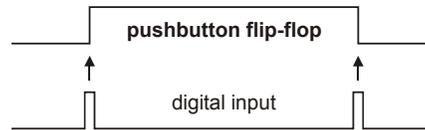
Fig. 3. Pushbutton for flip-flop characteristics
