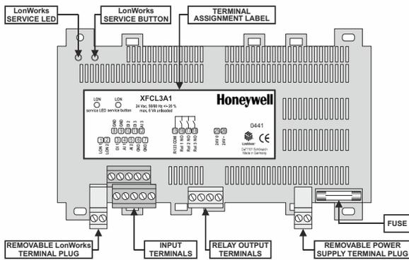
Fig. 2. Top view (optional terminal cover removed)
