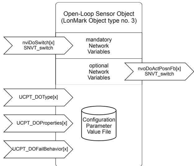
Fig. 9. Profile of LONMARK actuator objects for relays
