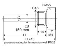
Fig. 6. TF21, TF31 immersion well dimensions (in mm)
