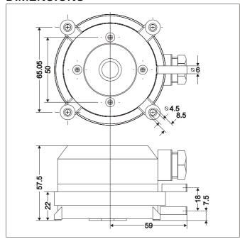
Fig. 3. Dimensions (in mm)
