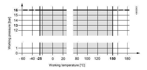
Working pressure and medium temperature staged as per ISO 7005
