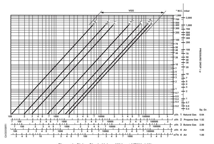
Figure 4. Sizing Single Valves Without NEMA 4 Kit.
