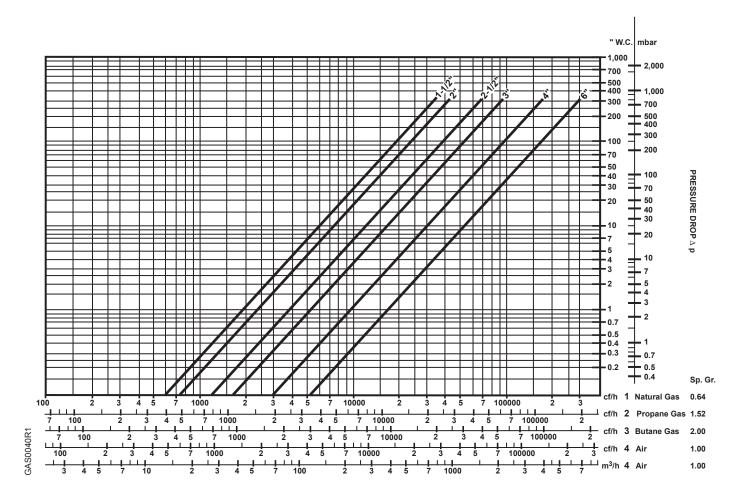
Figure 5. Sizing Double Valves.
