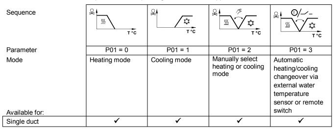
In application "Single duct with el. heater", the controller operates in heating AND cooling mode.
