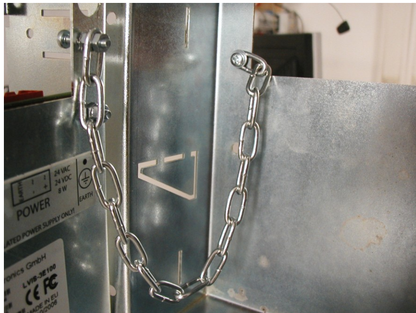
Figure 1: Connecting L-VIS to the wall mount frame.
