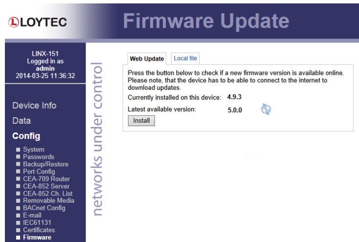
Figure 37: Firmware upgrade via the Web interface.
