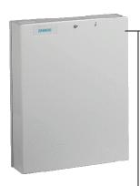
A large assortment of plug-in modules and peripherals such as LCD keypads, addressable expanders for inputs and outputs, card readers or external power supplies are available for professional installation. The panel feeds, controls and monitors the modules via E-Bus, which can be installed in any topology in the building.
