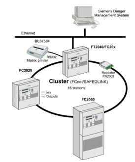
Using a fiber-optic Backbone (FCnet/LAN) up to 14 of the above mentioned clusters (with up to 16 stations each) can be networked. The entire network may contain up to 64 stations.
