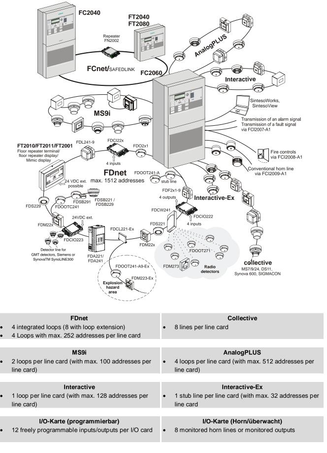
Mixed usage possible, but with a max. of 5 cards per control panel.
