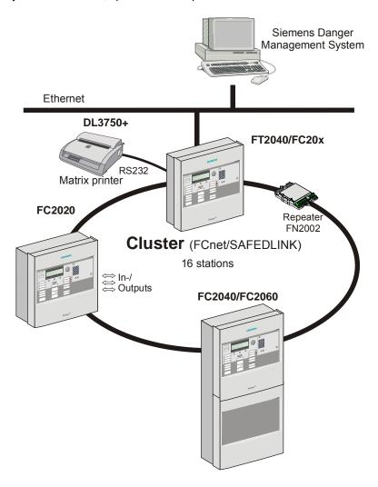
An optical Ethernet network (FCnet/LAN) allows up to 14 clusters with up to 16 stations to be operated on one network. A maximum of 64 stations is supported in total.
