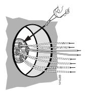
Comply with the various regulations on separating various voltage levels, when mounting the temperature sensor (with low voltage protection) alongside the recessed conduit boxes connected to the low-voltage power. In this case, the mounting frames must be connected to the protective ground wire with a flat plug connector plug and therefore grounded.
