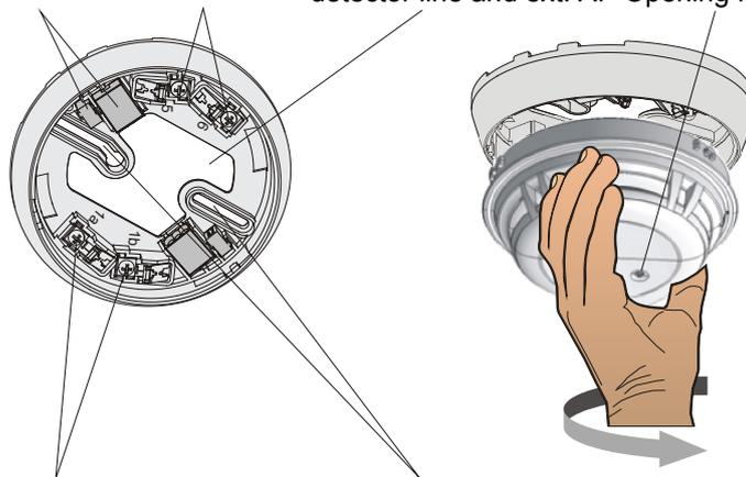
Connecting terminals detector line and ext. AI
