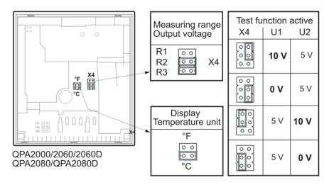
Measuring range R1 0 0 R2 0 0 00 R3 Output voltage °F 0 0 X17 R5 ໂດດີ R6 Display Temperature unit **QPA1000** °F QPA2002/QPA2002D 0 0 QPA2062/QPA2062D 0 0 °C
