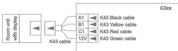
The room units communicate with the control unit via ZoneBus communication. The cable between the room unit and control unit should be a K43 cable which has a modular contact for the room unit. The cable can be ordered in different lengths up to 20 meter.
