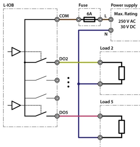
Figure 71: 6A relays with one external fuse
