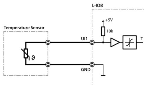
Figure 69: Temperature measurement on UI
