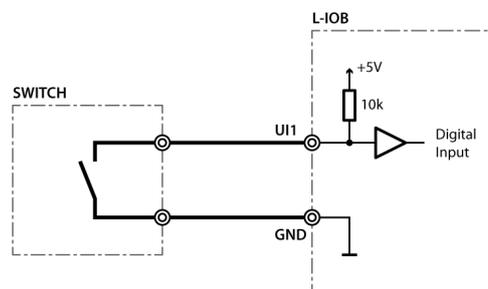
Figure 63: Switch connected to UI
