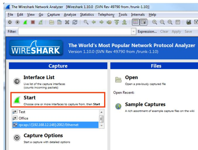
Figure 59: Start Remote Capture in Wireshark.
