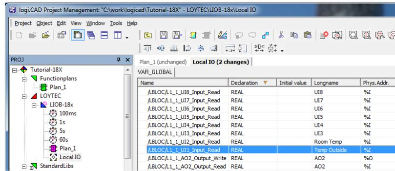
Figure 14: Exposed PLC data points appear in LogiCAD
