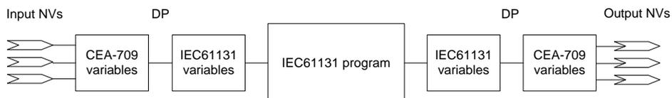
Figure 23: Usage of data points in IEC61131
