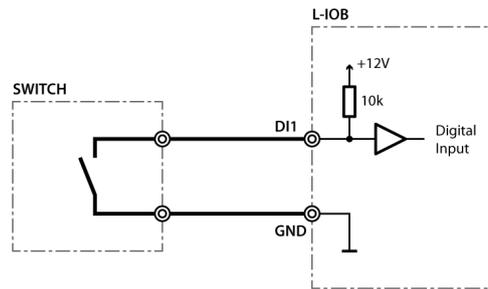
Figure 62: Switch connected to DI
