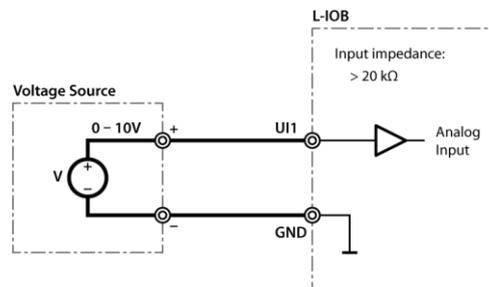
Figure 65: Voltage source on UI in analog mode
