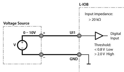
Figure 66: Voltage source on UI in digital mode
