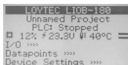
Figure 6: Main Screen of the LCD UI
