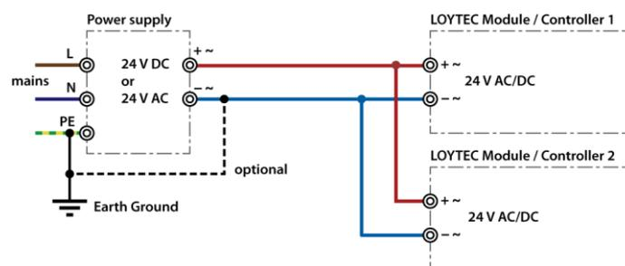
Figure 61: External power supply
