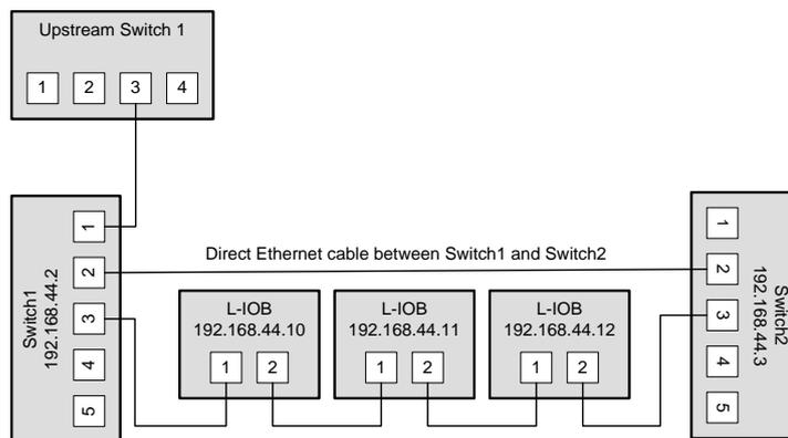
Figure 80: Single upstream connection.
