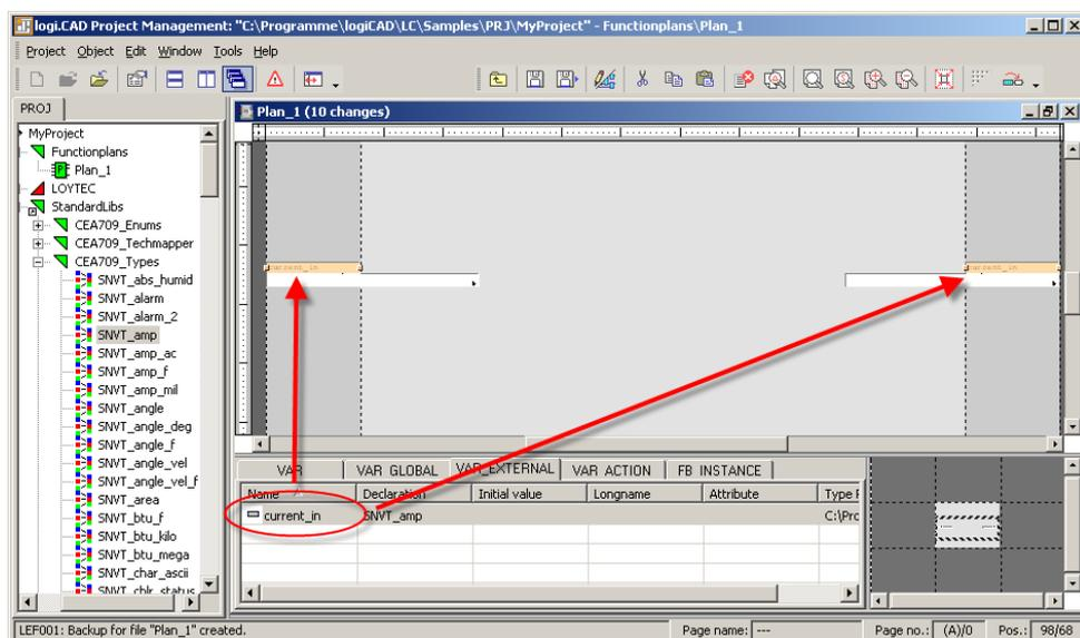
Figure 44: Drag-and-drop external variable to drawing area
