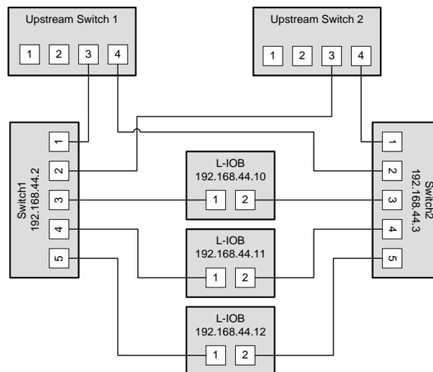
Figure 78: Fully redundant Ethernet topology
