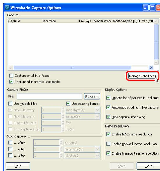
Figure 55: Wireshark Capture Options Dialog.
