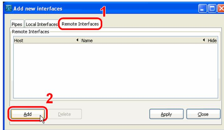
Figure 56: Wireshark Add New Interfaces Dialog.
