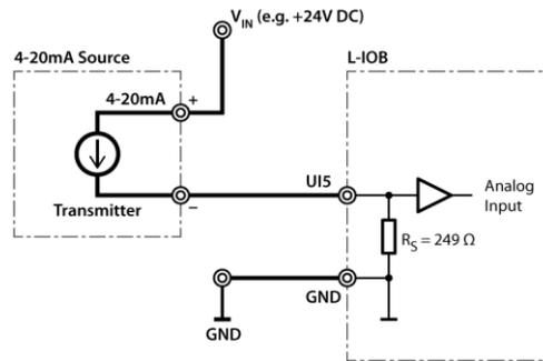
Figure 67: 4-20mA transmitter with internal shunt on UI
