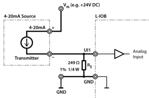
Figure 68: 4-20mA transmitter with external shunt on UI
