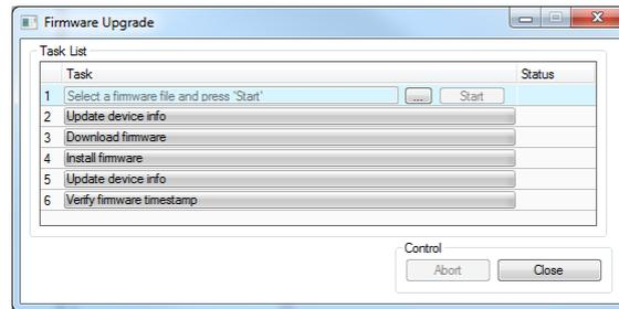
Figure 53: Firmware Update dialog of the Configurator
