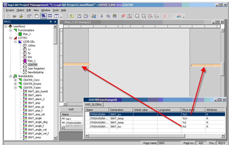
Figure 39: Adding global variables to Functionplans
