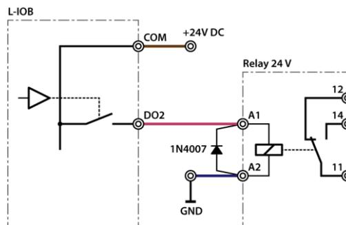
Figure 74: Suppressor circuit with free-wheeling diode
