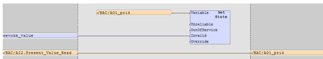
Figure 52: PLC with BACnet objects
