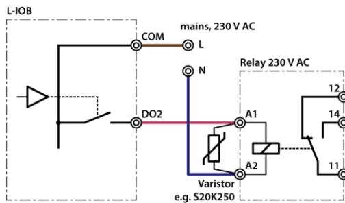
Figure 75: Suppressor circuit with varistor
