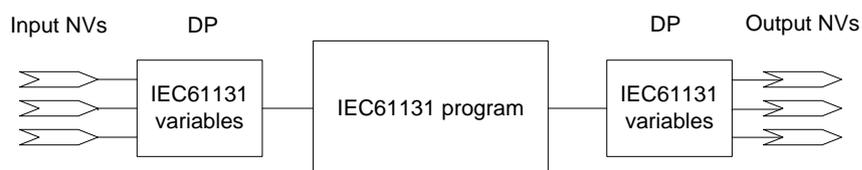
Figure 30: Connecting IEC61131 variables
