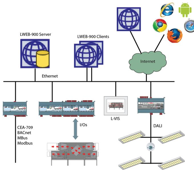
Figure 2: LWEB-900 System Architecture
