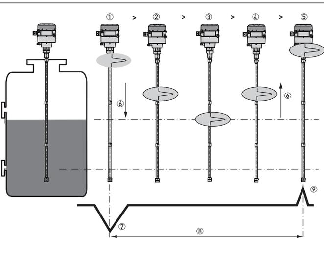
The AKS 4100/4100U electronic converter emits low-intensity, high frequency electromagnetic pulses with a width of approximately 1 nanosecond, which travel at the speed of light along the probe (wire or coaxial cable) down to the liquid surface.
