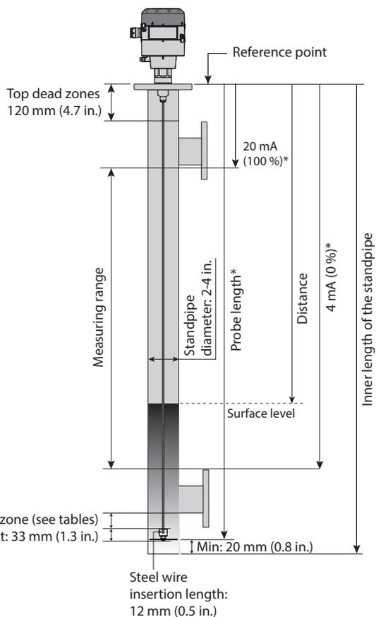
\* Values to be entered into HMI Quick Setup menu and recorded on the setting label. Stick the setting label onto the Signal Converter either inside or outside.
