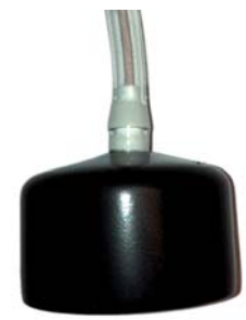
Calibration Cup Assy, IR-RS Cup Inner Diameter: 42.8mm Tubing Inner Diameter: 5mm Note: The cup has four equal cuts to allow it to fit over the IR-RS sensor as shown below. Usage: IP41 units with IR-RS sensor
