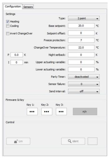
**Controller Type** can be set to 2-point control or proportional control (PI-loop) with PWM for thermal actuators.
