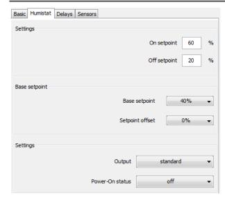
Humidistat application is a 2-point control of the relative humidity using a rH-sensor (EEPs: A5-04-01 or A5-10-10/11/12)
