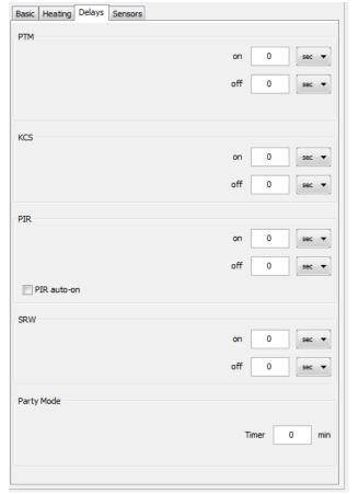
For all sensor types: An ON- and OFF-delay can be set from 0..99 sec or 0..99 minutes.
