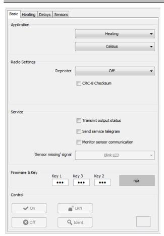
In the 1<sup>st</sup> tab "Basic", the "Application" must be selected using the drop down menu. Depending on the selected application airConfig will offer additional tabs to configure the device.
