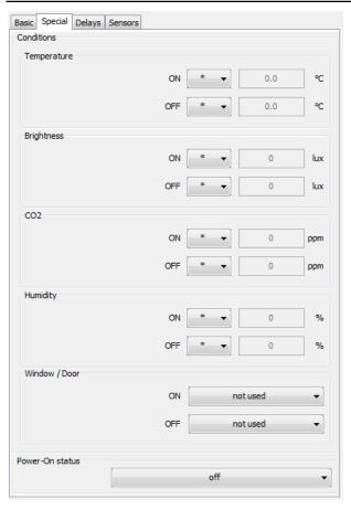
Custom programmable applications using 2-point control based on temperature, brightness, CO2, relative humidity or window status. Custom programs can be selected: "more – less – equals" can be selected in combination with a threshold to turn on or off the relay.
