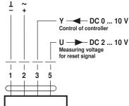
Override control (Frost protection circuit)
