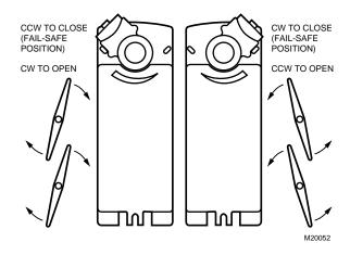
Fig. 2. Spring Return DCA mounting orientation.
