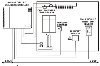
⚠ Digital wall module T7560B has internal humidity sensor.
