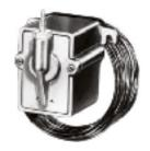
One-pipe, direct-acting temperature sensor used with RP920 controllers to provide proportional control of pneumatic valve or damper actuators. Averaging, liquid filled element for duct mounting. Easily formed into variety of configurations to assure sensing of average temperatures.
