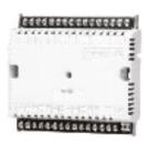
The W7761A is the remote input/output (RIO) device in the Excel 10 product line family. The RIO is a LonMark compliant device designed to monitor/control HVAC equipment, lighting and other miscellaneous loads in a distributed network or with a zone manager. Uses Echelon LonWorks networks protocol. Designed for floating and PWM control, and for remote connection of various actuators.
