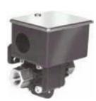
Differential pressure switch for water or air. Opens or closes the switch contact in response to a change in sensed differential pressure. Suitable for pump and filter applications.
