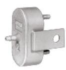
A three port relay used in HVAC systems, averages the signals from two thermostats to control a single device such as a heating coil valve for a multi-zone unit. The pneumatic averaging relay provides an output pressure equal to the average of the two input pressures.
