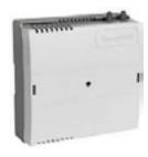
Variable Air Volume (VAV) controller in the Excel 10 family. Using single and dual duct application these VAV systems provide pressure independent or pressure dependent air flow control and series or induction fan control. VAV systems generally provide cool air only to the zones. The W7751 controllers provide additional outputs that control VAV box reheat coils. The heaters can be staged electric or modulating hot water. Supply and exhaust pressurisation control are provided on a zone basis.
