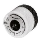
A four port, non-bleed pneumatic relay which produces a modulating pressure output, proportional in a fixed ratio to pilot input changes. Controls pneumatic valve or damper actuators in sequence from a single thermostat.
