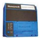
Microprocesser-based integrated flame switch for detecting a flame using rectification, ultraviolet (UV) or infrared (IR) source. Provides level of safety, functional capability and features beyond conventional controls. Use with flame signal amplifiers R7847, R7848, R7849, R7851, R7861 or R7886
