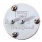
Three port relay used in HVAC systems to perfom a variety of relay functions; tranmit the higher of two input signals, lock out one pressure signal when second signal is higher, or tranmit the lower of two pressure signals.
