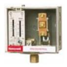
L404F Pressuretrol controllers provide operating control with automatic limit protection for pressure systems of up to 2070Kpa or 300psi. Mounting 1/4" NPT Internal thread or surface mount through back of case. Switch operation Auto recycle
