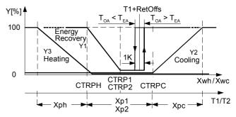
A fixed hysteresis of 1K is used, to switch between 0% position and actual Y1 signal.
