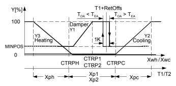
A fixed hysteresis of 1K is used, to switch between **MINPOS** and actual Y1 signal.
