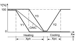
Sequence control with one output for heating and two outputs for cooling (YMode = 3)
