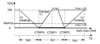
Note: If the R7426B controller with floating output is used for mixed air damper control, care must be taken, that the output load of maximum 450mA is not exceeded.
