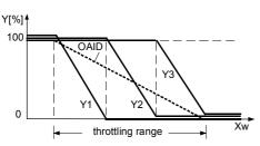
Sequence control with two outputs for heating and one output for cooling (YMode = 2)
