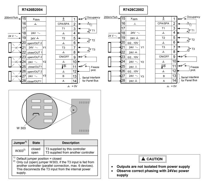
Fig. 3. Connections and Jumper coding
