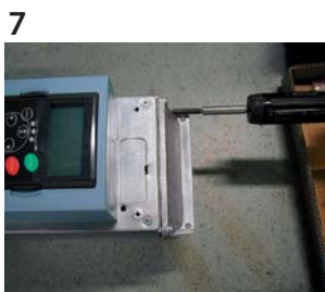
7 Fix the top flange to its place.
