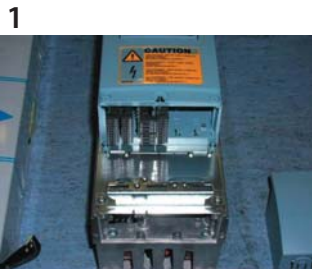
1 Open the control cable cover and remove the cable entry flange
