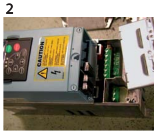
2 Detach the protection plate. Keep the plate and the screws to hand, they will still be needed.
