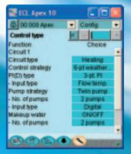
Configuration of control functions where the functionality of each heating circuit can be configured for individual control functions.
