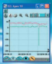
One week of data logging in a heating circuit. The log probes are: Outdoor temperature, flow temperature and flow reference.
