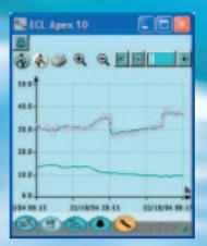
12 hours of data logging in a heating circuit. The log probes are: Outdoor temperature, flow temperature and flow reference.
