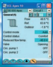
The primary parameters and sensor values of the heating circuit.
