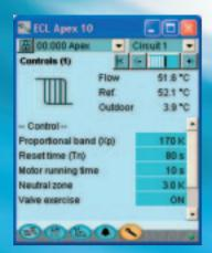
Adjustment of control parameters where each parameter has a short description and the actual value is shown. The primary values of the heating circuit are shown in the top of the window.
